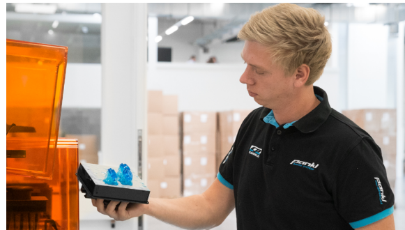
Process engineer Christian Joebstl runs three Form 2 SLA 3D printers in Pankl's production facility.
